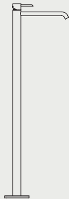
Floor mounted single lever basin mixer: Without pop-up waste set. "Plus" aerator. Cold-water opening. Monomando lavabo instalación a pavimento.
